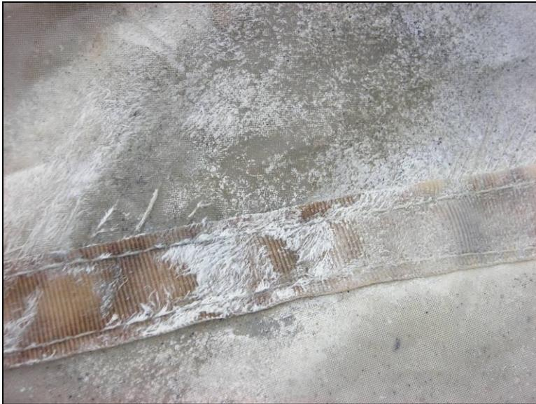
Figure 93. White filamentous material on net at Von Ormy Growers Well.
