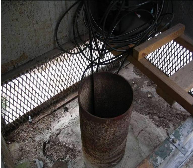
Figure 34. A bottle trap was used to sample the City of Kyle well, located underneath the Kyle water tower.
