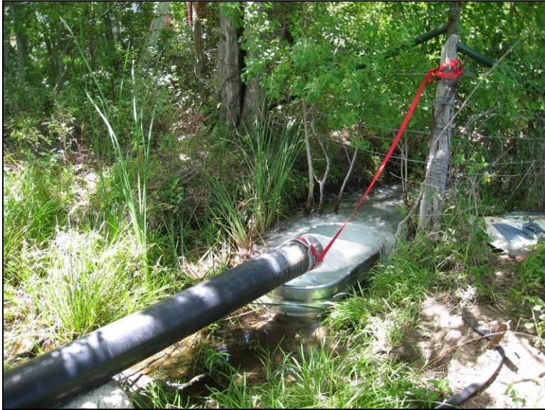
Figure 90. The initial sampling setup at the Verstuyft Home well involved flowing water through a net into a metal tub to keep the net submerged.
