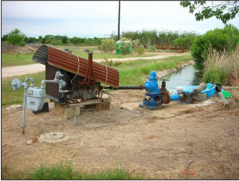
Figure 92. A plastic pool was placed underneath the outlet from the Von Ormy Growers Well to keep the net submerged when the discharge was not flowing into the irrigation canal.
