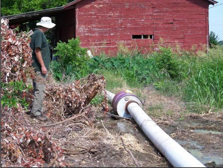
Figure 42. In-line barrel sampler at the Homer Verstuyft Well.
