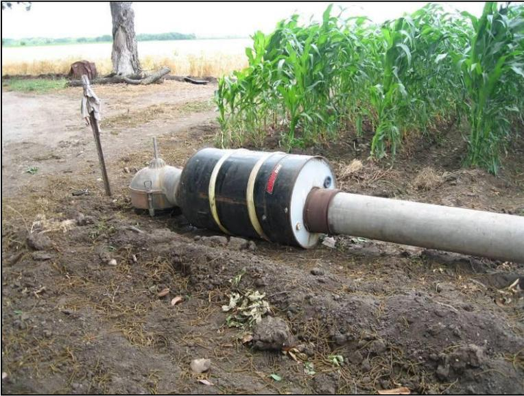
Figure 53. The east outlet of the Loop 353 Well is fitted with an in-line sampler.
