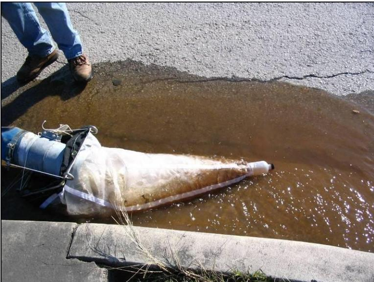
Figure 50. A plankton net secured to the end of the net captures outflow from the LCRA well.
