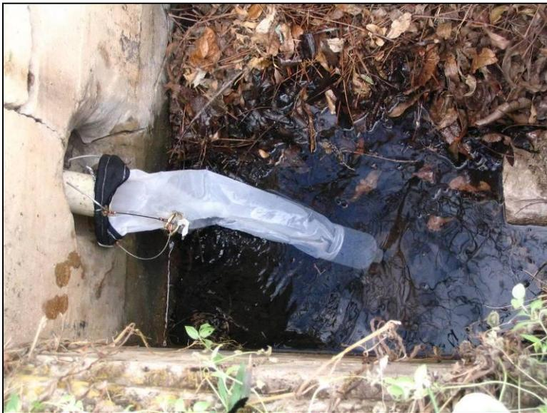
Figure 36. A plankton net was attached to the outflow at FSH #2. The collection bottle remains submerged when there is water pooled in the drain.
