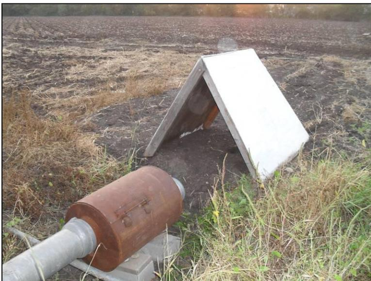
Figure 52. A closed barrel sampler was installed on the west outlet of the Loop 353 Well in 2010.
